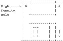
As a temporary workaround, place a small piece of tape over both sides of the extra hole (the one on the upper left when looking at the diskette from the front, as shown in the above diagram) on the high-density disk to trick the Macintosh into treating the disk as a double-density disk. This is a temporary solution, and the tape should be removed and the disk reformatted to the proper size as soon as possible.
