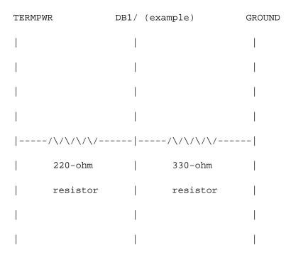
The obvious tradeoff here is cost versus time to build this terminator. It would seem that size is also an issue; this is a lot of resistors and solder joints to deal with.
