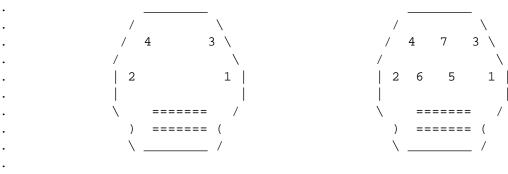
4-pin S-Video Connector Apple 7-Pin S-Video Input Connector
