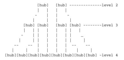
Whether the cascaded hub configuration is a better design than the backbone depends on several factors.
