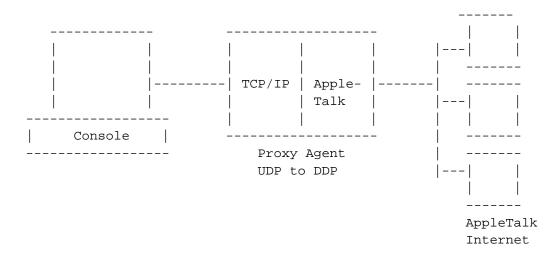
Other types of Proxy Agents can be used in SNMP networks. For example, Proxy Agents can sit on a network and monitor packet traffic, gather statistics, and send traps to consoles when certain conditions occur.
