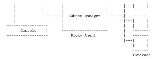
This Proxy Agent has the added advantage of cutting down on network traffic, and frees the console from having to monitor a large number of nodes on a one-to-one basis. Subnet managers are under development by several vendors.
