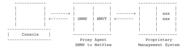
In the case of nodes that do not understand TCP/IP, but do support SNMP, a Proxy Agent can strip out the SNMP-specific data units and encapsulate them in another transport. A more complicated function of this type of agent is
