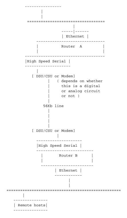
Note: Router A and router B must speak a compatible protocol over the high-speed serial connection.
