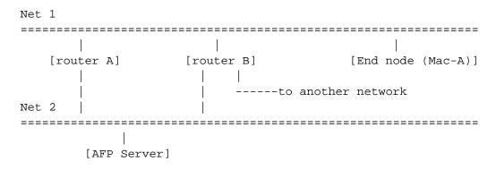
In this case, either router A or router B would work as the "best route" to network 2. In detail:
