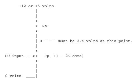
The voltage range at the GC inputs should go from 0v to 2.4v. The value of Rs can be calculated for +5 volt systems with this formula:
