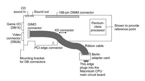
Figure 3-1 Locations of I/O connectors for the 12" card
