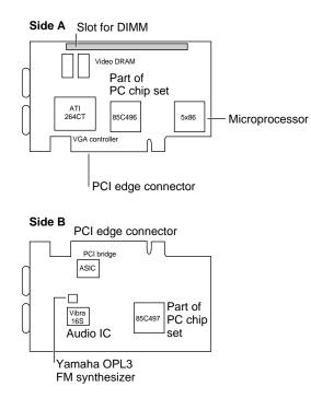
Note: PCI edge connector is shown to define orientation.
