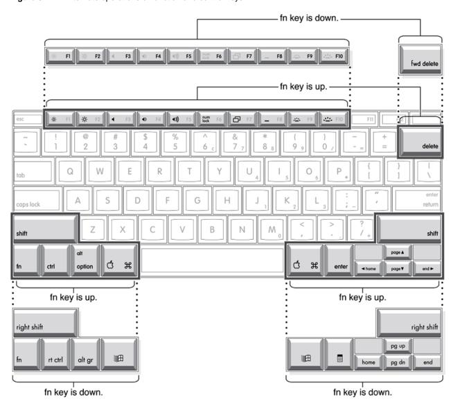
Figure 3-8 Embedded numeric keypad operation
