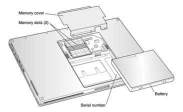
Figure 4-1 Removing RAM expansion slot cover
