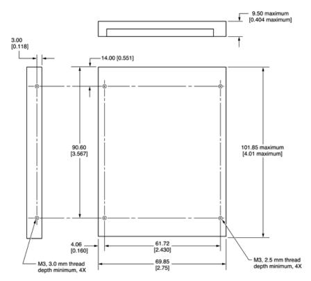
Note: Dimensions are in millimeters [inches].
