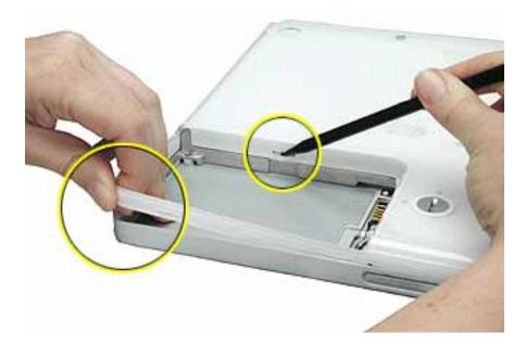
9. Starting at the battery compartment, use a black stick to carefully pry up the bottom case from the computer.
