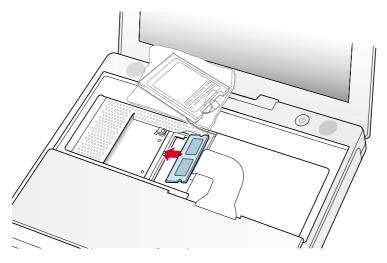
2. Gently push the top of the card down until the brackets snap onto both sides of the memory card to lock it into place (Figure 11).
