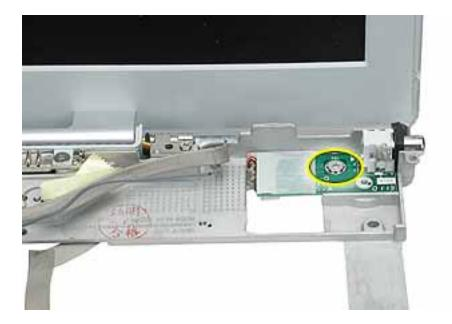
3. Tilt up the computer and note the routing of the flat power cable across the underside of the inner frame.
