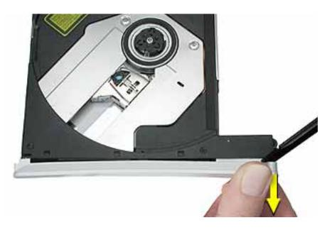
3. Use the flat end of the black stick to detach the middle tab and remove the door.
