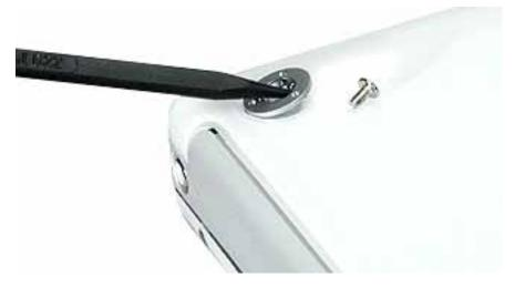
6. Remove the two Phillips screws next to the battery connector.
