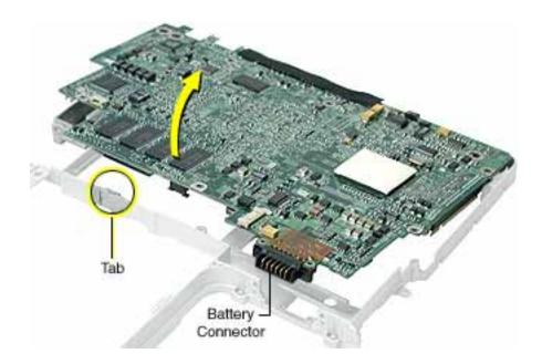
9. Install the replacement logic board, and reassemble and test the computer.
