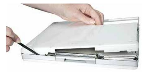
12. If you are replacing any additional parts at this time, remove the two springs from the battery compartment so they do not fall out and get lost.
