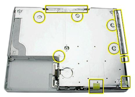
4. **Warning: Do not bend the bottom shield.** Lift the bottom shield off the computer, being careful where it might catch on the tape.
