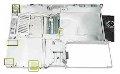
3. **Warning: Do not bend the top shield.** Lift the top shield off the computer, being careful where it might catch on the highlighted areas shown.
