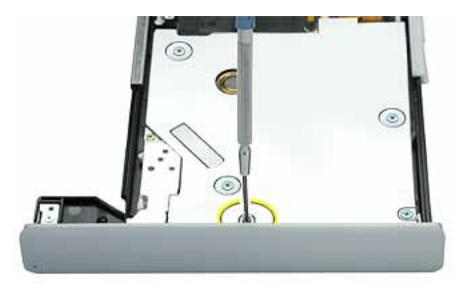
2. Press on the wide tab, and pull that end of the door away from the drive.
