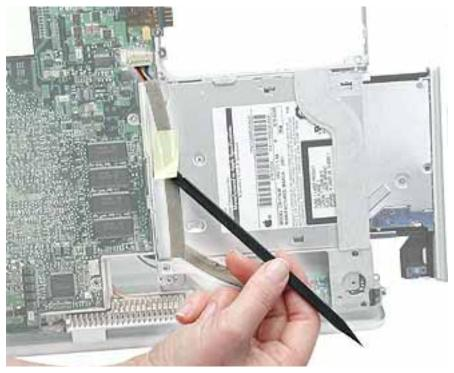
2. Remove the single screw from the DC board.
