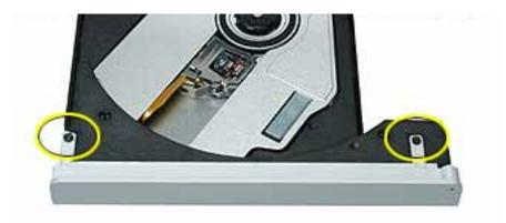
2. Gently tilt the door away from the screw holes to release the hooks underneath that hold the door in place.
