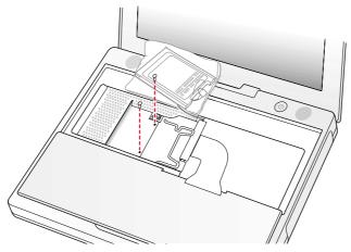
5. Lift the RAM shield out of the computer. Carefully pulling up on the wire holder may help to remove the shield (Figure 8).
