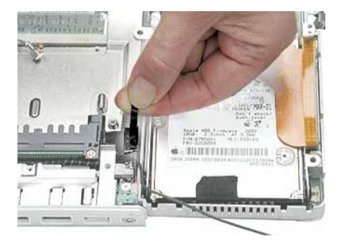
3. Peel the tape off of the optical drive, and disconnect the flat backlight cable from the logic board.
