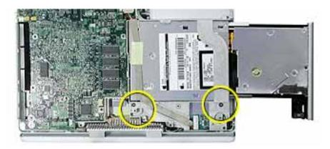
3. Note the routing of the flat power cable across the underside of the optical drive.Lift up the tape from the flat power cable.
