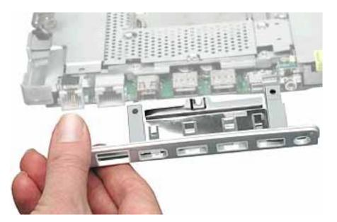
3. Install the replacement I/O bezel, and reassemble and test the computer.
