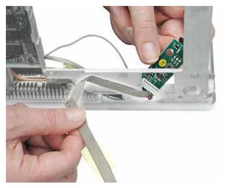
4. Install the replacement DC board, and reassemble and test the computer.
