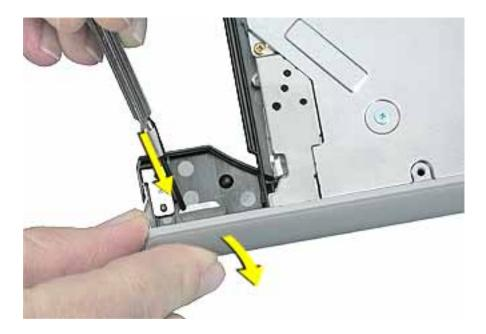
3. Release the tab at the other end of the door, and pull the door straight up to free it from the drive.
