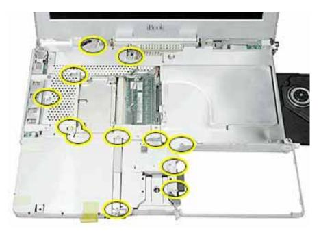
2. Using a black stick, carefully peel up, but do not remove, the two foil strips and three pieces of tape.
