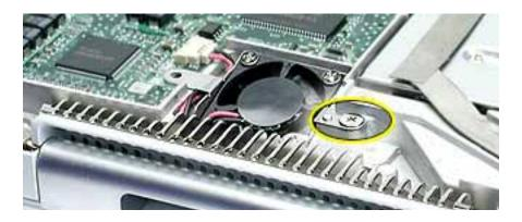
2. Lift the fan and bracket from the computer, and use a black stick to disconnect the connector from the logic board.
