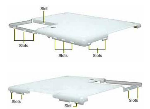
8. In the battery compartment, lift up the corner of the bottom case, and use a black stick to gently pry up the slot from the inner tabs on the frame.
