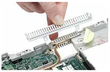
5. Remove the remaining screw at the heat spreader plate.
