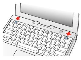
4. Flip the keyboard over and lay it on the palm rests and trackpad.
