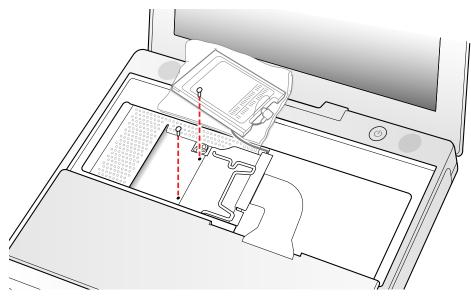
10. Lift the RAM shield out of the computer. Carefully pulling up on the wire holder may help to remove the shield.
