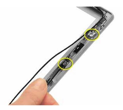
6. Tilt up the antenna receptor to remove it from the bezel assembly.
