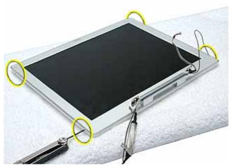
2. Using a black stick, pry up the bezel from the display housing. Carefully work the black stick around the outer perimeter and corners of the bezel.
