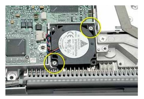
2. Lift the fan from the computer, and use a black stick to disconnect the connector from the logic board.
