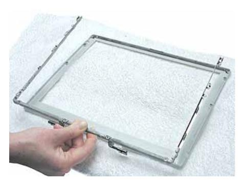
6. Install the replacement bezel brace with clutch assembly, and reassemble and test the computer.
