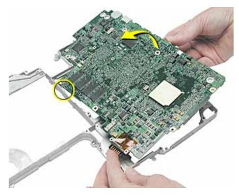
9. Install the replacement logic board, and reassemble and test the computer.
