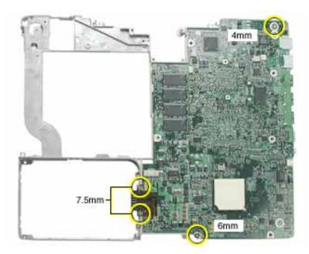
8. Lifting the logic board at the back ports, tilt up the logic board to remove it from the frame.
