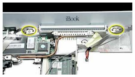
6. Warning: When lifting the display, be careful not to strain the cables.
