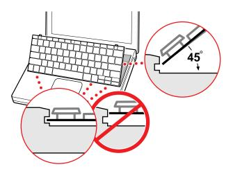
• Pull down on the keyboard release tabs and then press down on the top portion of the keyboard.
