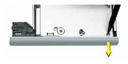
3. Press the wider tab, and pull the door off of the drive.
