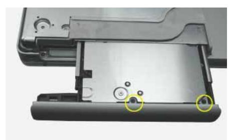
2. Press on the wide tab, and pull the door away from the drive.
