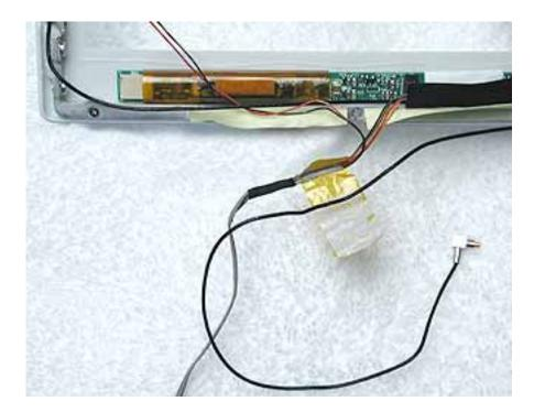
5. Disconnect the data cable from the inverter board at CN1.
