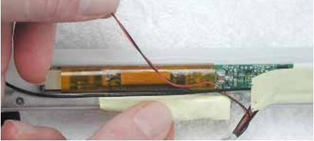
4. Warning: When removing the tape that bundles the reed switch cable assembly to the AirPort Card antenna cable, be careful not to strain or pinch the cables.
