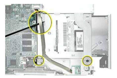
4. Tilt back the computer, and on the other side of the optical drive, loosen the tape holding the backlight cable to the optical drive. Reserve the tape for installation of the replacement drive. Do not disconnect the backlight cable.
