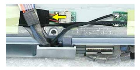
6. Remove the reed switch cable assembly.
