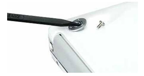
6. Remove the two identical Phillips screws next to the battery connector.
