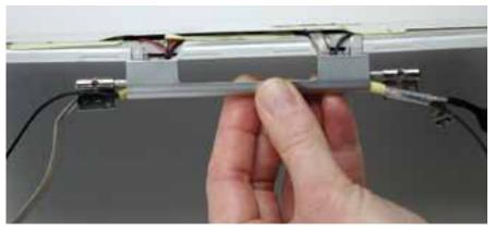
**Note:** The clutch caps are mirror images of each other. There is a right clutch cap and a left clutch cap. Note the positioning of the clutch caps on the display clutch cover. The image below shows the left clutch cap installed.
