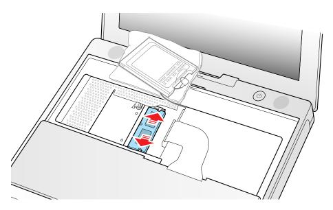
3. Line up the notch in the replacement memory card with the small tab in the memory slot. Hold the card at a 30-degree angle, then push the card into the slot until it is firmly seated.
