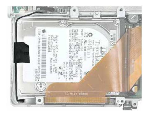
2. Pull up the flexible tab to disconnect the LVDS (low voltage data signal) cable from the logic board.
