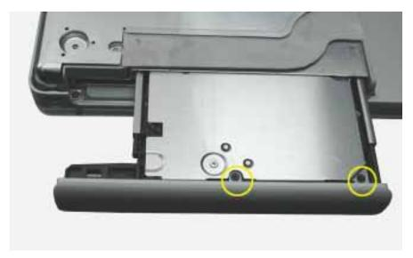
2. Press on the wide tab, and pull the door away from the drive.
