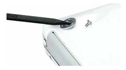
6. Remove the two identical Phillips screws next to the battery connector.
