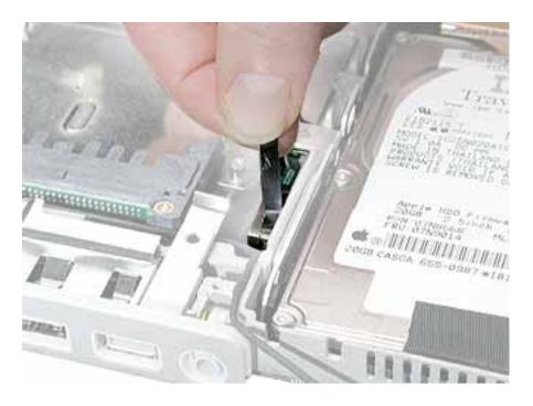
3. Peel the tape off of the optical drive, and disconnect the flat backlight cable from the logic board.
