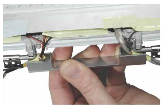
**Replacement Note:** When installing the replacement clutch cover, hold the cables and clutch cap in place as you slide the clutch cover over them.
