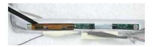
**Replacement Note:** The inverter board is held to the bezel assembly with double-sided tape on each end of the board. Use new double-sided tape when installing the replacement inverter board.
