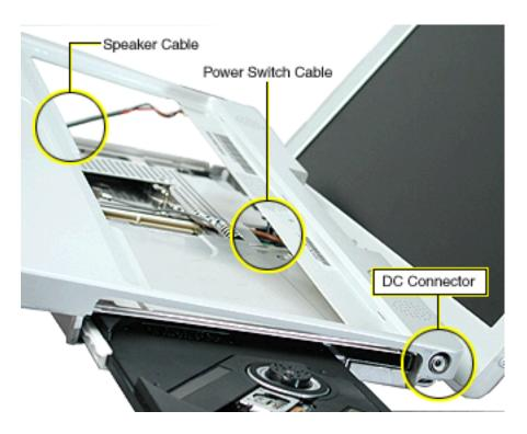
9. With the top case loosened, note how the speaker cable is routed.
