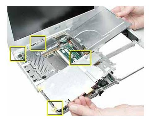
4. Install the replacement top shield, and reassemble and test the computer.
