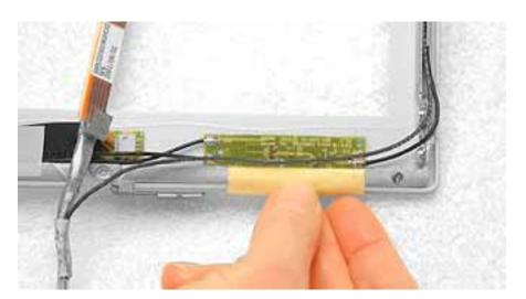
3. Warning: When lifting the antenna board, be careful not to strain or pinch the cables.
