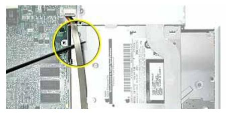
Tilt up the computer and note the routing of the flat power cable across the underside of the inner frame.
