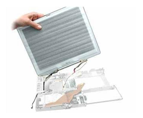
7. Warning: While supporting the display, do not tug on the remaining cables. Make sure the cable insulation is not torn or damaged.
