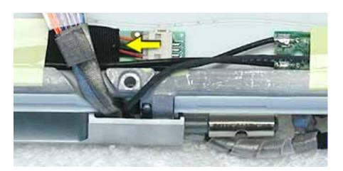
6. Remove the reed switch cable assembly.
