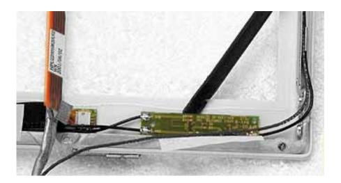
4. With the antenna board loosened, note the cable routing on each side of the bezel. On the right, the antenna receptor cable is routed underneath the microphone cable through two channels before terminating at the receptor bracket.
