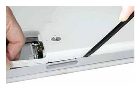
10. Warning: To avoid damaging the sleep light and other delicate components, do not insert the black stick too far into the computer as you free the bottom case from the computer. Use just the tip of the black stick to pry up the bottom case.
