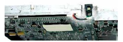
2. Using a black stick, disconnect the sleep light board connector from the logic board.
