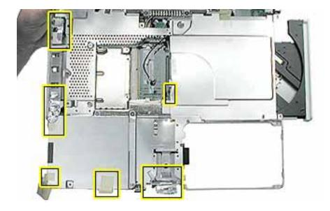
3. Lift up the foil tape near the trackpad cable.
