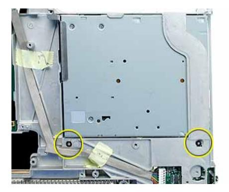
8. Turn the computer upright, and without straining the backlight cable, loosen the tape that secures the cable to the computer frame.
