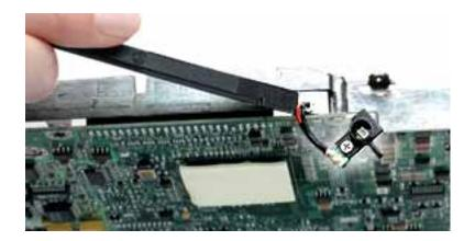
3. Remove the screw from the reset button board, and disconnect the connector from the logic board.
