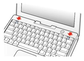
9. Flip the keyboard over and lay it on the palm rests and trackpad (Figure 4).
