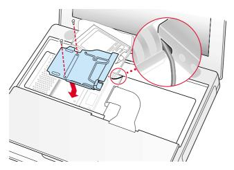
7. If you do not have an AirPort Card, flip down the wire holder over the AirPort Card antenna cable and secure it by inserting the prongs of the holder into the slots in the RAM shield (**Figure 13**).
