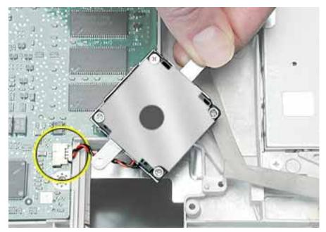
3. Install the replacement fan, and reassemble and test the computer.
