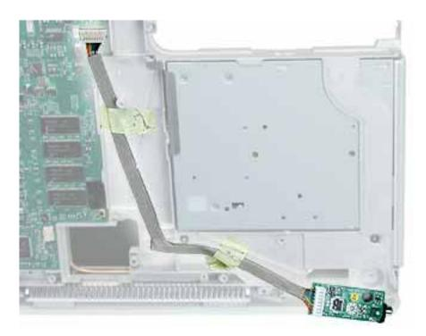
5. Install the replacement DC board, and reassemble and test the computer.
