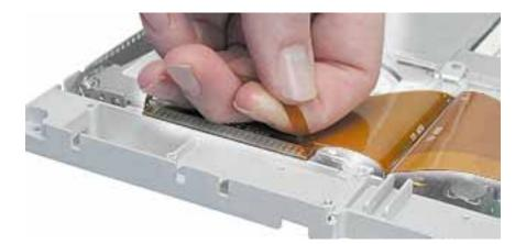
4. Lift up the fabric tape to release the microphone cable.
