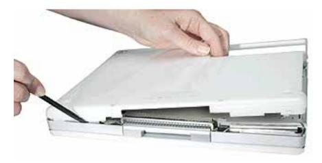
14. If you are replacing any additional parts at this time, remove the two springs from the battery compartment so they do not fall out and get lost.
