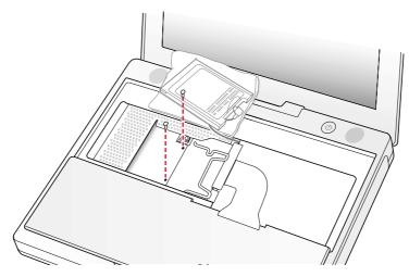
5. Lift the RAM shield out of the computer. Carefully pulling up on the wire holder may help to remove the shield (Figure 8).
