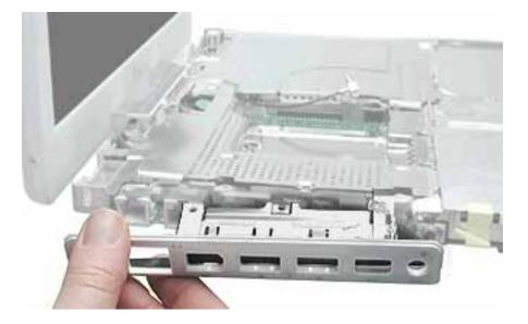
3. Install the replacement I/O bezel, and reassemble and test the computer.
