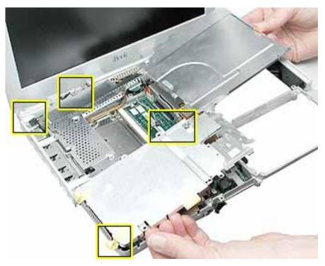
6. Install the replacement top shield, and reassemble and test the computer.
