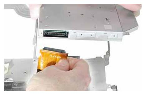
13. Install the replacement optical drive, and reassemble and test the computer.
