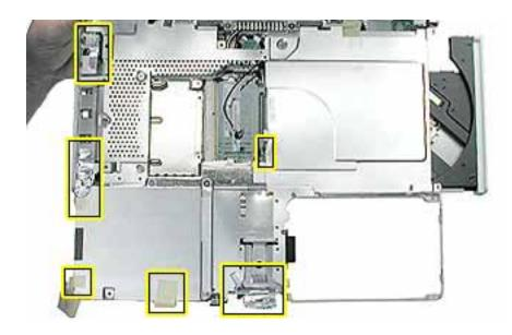
3. Lift up the foil tape near the trackpad cable.
