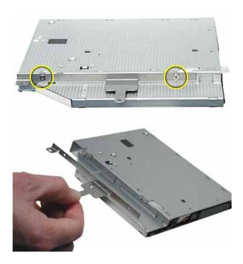
14. Install the replacement optical drive, and reassemble and test the computer.
