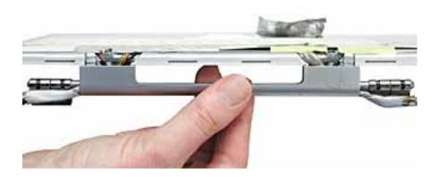
**Note:** The clutch caps are mirror images of each other. There is a right clutch cap and a left clutch cap. Note the positioning of the clutch caps on the display clutch cover. The image below shows the left clutch cap installed.
