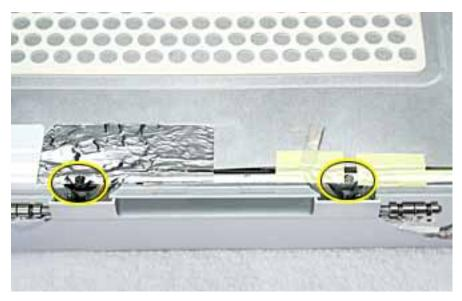
10. Loosen the remaining tape that secures the shield to the assembly. Remove the shield.
