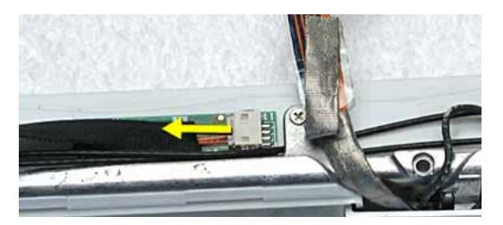
6. Remove the reed switch cable assembly.
