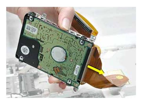
7. Holding the drive by the corners as shown, pull off the side rails (with grommets attached).
