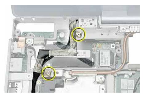
6. Peel the tape off of the computer frame, and disconnect the flat backlight cable from the logic board.
