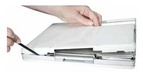
14. If you are replacing any additional parts at this time, remove the two springs from the battery compartment so they do not fall out and get lost.
