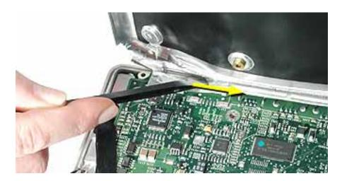
5. Note: The two springs in the battery connector can become loose. When reassembling the computer, make sure that the two springs in the battery connector are in place before installing the bottom case. Each spring might have grease on the coils, and each has a plastic cap on one end. Make sure the cap fits securely on the spring, and the curved side of the cap is positioned against the inner frame.
