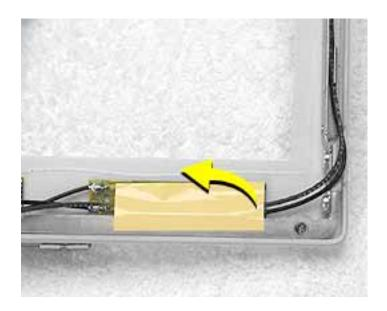
3. Warning: When lifting the antenna board, be careful not to strain or pinch the cables.
