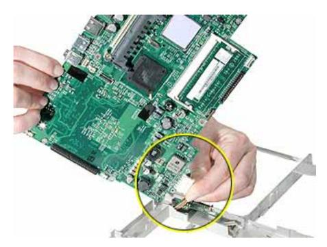
12. Install the replacement logic board, and reassemble and test the computer.
