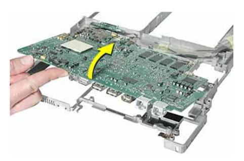
11. Disconnect the logic board from the battery transfer board connector.
