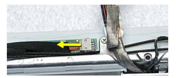
6. Remove the reed switch cable assembly.
