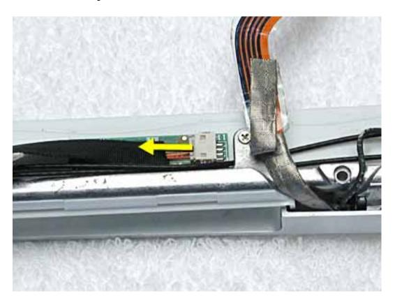
2. **Replacement Note:** Note the position of the inverter board and cables for the installation of the replacement inverter board.
