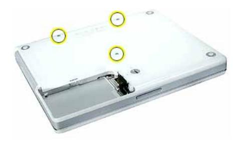
3. Using a black stick, peel up the three rubber feet from the metal sockets.
