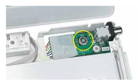
2. Tilt up the DC board and route it through the opening in the computer frame.
