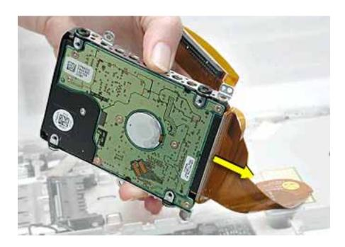
7. Holding the drive by the corners as shown, pull off the side rails (with grommets attached).
