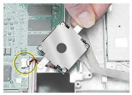
3. Install the replacement fan, and reassemble and test the computer.
