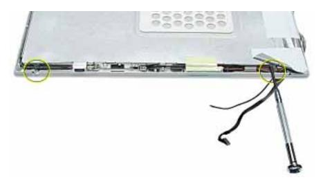
7. Peel up the foil tape that holds the LCD cable to the LCD shield.
