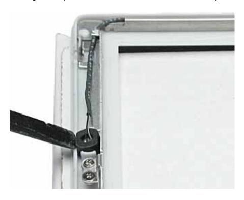
3. Working around the perimeter of the bezel, pull up the microphone cable from the cable channel, being careful not to strain any other cables.
