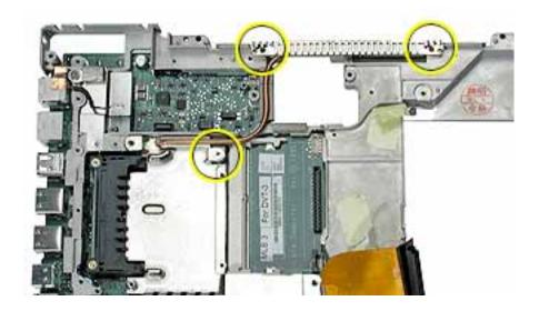
6. Tilt up the heat spreader and lift it off the logic board and out of the frame.
