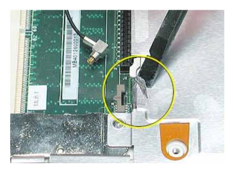
4. Before lifting up the top shield, note that the shield fits over posts on the computer frame.
