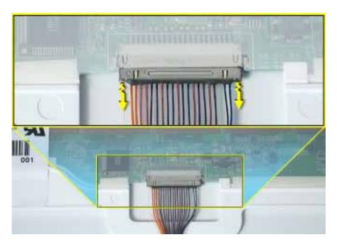
12. At the other end of the LCD cable, remove the tape from the bottom edge of the LCD panel.
