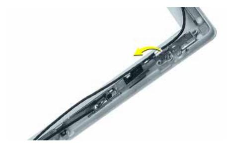
9. On the left side of the bezel, remove the two 3-mm long Phillips screws at the antenna receptor.
