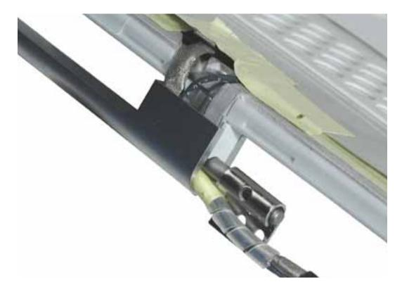
Make sure the clutch cap on each side of the clutch cover is firmly seated before installing the two screws.
