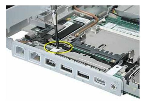
2. Tilt down the I/O bezel and remove it from the computer frame.
