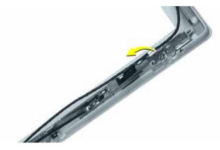
9. On the left side of the bezel, remove the two 3-mm long Phillips screws at the antenna receptor.
