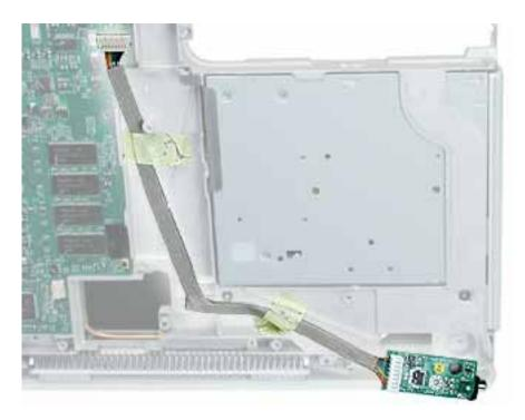
5. Install the replacement DC board, and reassemble and test the computer.
