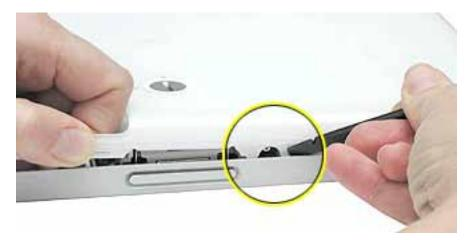
11. Carefully work the black stick around the corners of the bottom case.
