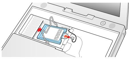
Use the wire holder to secure the AirPort Card in place by inserting its prongs into the slots in the RAM shield.
