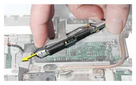
7. Install the replacement modem, and reassemble and test the computer.
