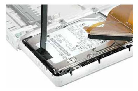
5. From the corner bracket, tilt up the hard drive, and slide it out from under the microphone cable.
