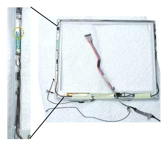
3. Lift up the cables and peel up the tape that covers the cables running along the bottom of the inverter board.
