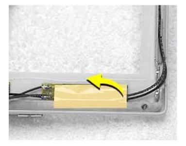
3. Warning: When lifting the antenna board, be careful not to strain or pinch the cables.
