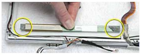
3. Install the replacement inverter board, and reassemble and test the computer.
