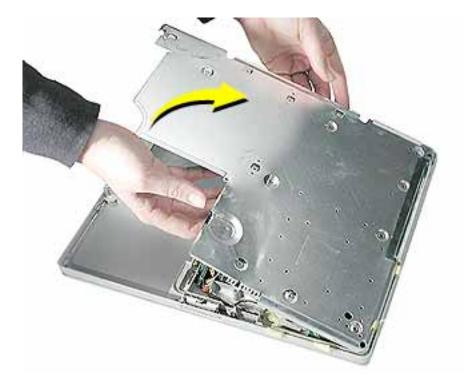
4. If necessary, use a black stick to separate the foil tape on the bottom shield from the I/O bezel shield.
