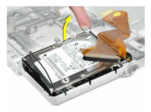
6. Warning: Handle the hard drive at the sides only. Do not touch or press anywhere else on the drive.
