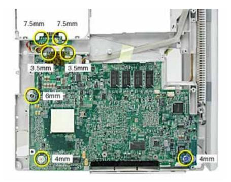
**Note:** When reassembling the computer, make sure that the underside of the replacement logic board includes the thermal transfer pad covering the large chip.
