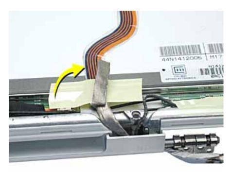
13. Warning: When lifting the LCD panel, be careful not to strain the inverter cable.
