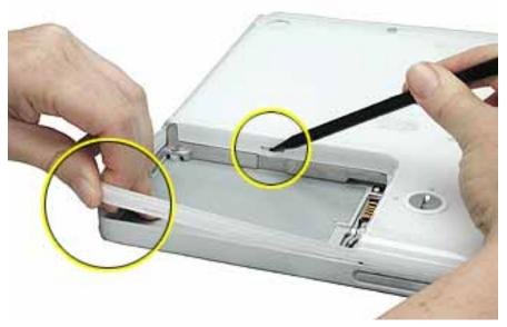
9. Starting at the battery compartment, use a black stick to carefully pry up the bottom case from the computer.
