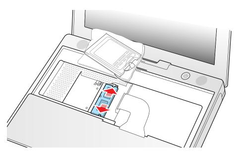
3. Install the replacement memory card by lining up the notch in the memory card with the small tab in the memory slot. Hold the card at a 30-degree angle, then push the card into the slot until it is firmly seated.
