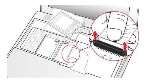
14. Install the replacement keyboard, RAM shield, and AirPort Card (if used).
