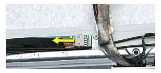
6. Remove the reed switch cable assembly.
