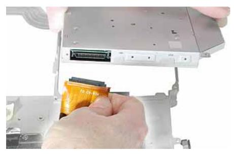
13. Install the replacement optical drive, and reassemble and test the computer.
