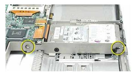
**Important:** When the rubber stoppers are inserted, push down on all four corners of the drive to verify that the drive is level and secure.
