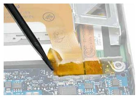
11. Remove the Kapton tape from the two-pin power switch connector at the right corner of the logic board. Disconnect the two-pin connector.
