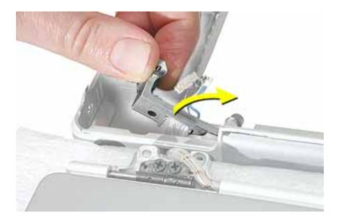
3. Warning: The LVDS cable and connector are extremely delicate. Do not pull or pinch the LVDS cable or connector. If necessary, use a black stick or other nonconductive tool to guide the cables out of the top case.
