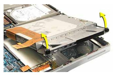
**Note:** There are four rubber stoppers (two on each side) on the DVD-ROM drive that fit over metal posts at the corners of the drive. Remove any that may have fallen off inside the computer.
