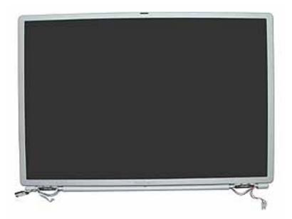
6. **Important:** When the replacement display module is installed, and before the clutch covers are installed, test that the display is seated properly. With the computer upright and closed, press the computer latch. The display module should pop up slightly if the module is properly seated.
