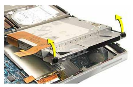
**Note:** There are four rubber stoppers (two on each side) on the drive that fit over metal posts at the corners of the drive. Remove any that may have fallen off inside the computer.
