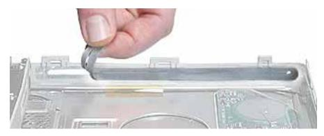
Apply the new felt strip to the slot-load area. Make sure the new felt strip lies flat. Use a black stick to run the length of the slot to make sure that the felt strip does not block any of the slot.
