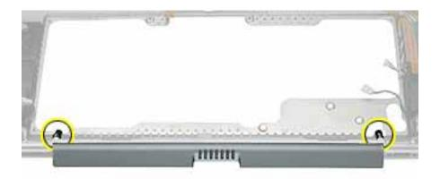
2. Lift off the inner clutch mounts, and pull door away from the top case.
