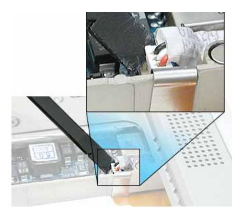
4. Disconnect the shielded, 3-pin backup battery connector from the logic board.
