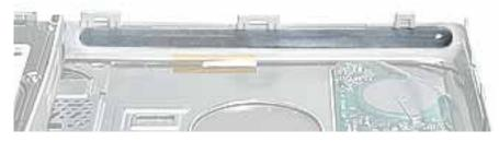
Peel off the felt strip from the inner top case. If there is any residual adhesive on the top case, rub it away.
