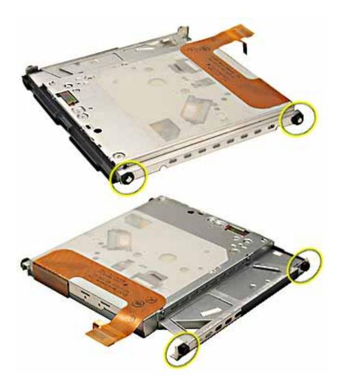
5. Warning: To prevent damage to the optical drive, handle the drive only by the corners. Do not press on the body of the drive.
