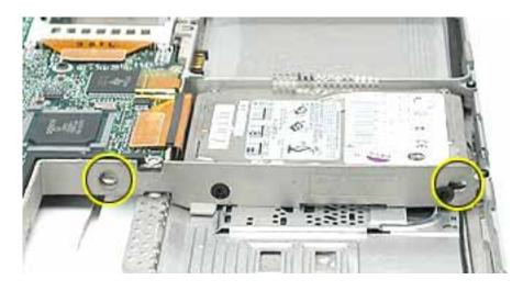
**Important:** When the rubber stoppers are inserted, push down on all four corners of the drive to verify that the drive is level and secure.
