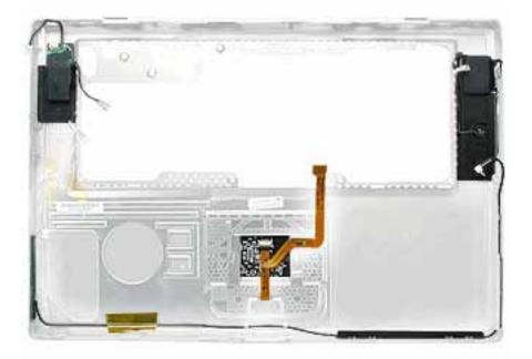
3. **Important:** Make sure you transfer the original serial number label from the old top case to the serial number panel on the replacement top case. You can use a black stick to carefully peel up a corner of the label. Then peel off the label completely and apply it to the serial number panel. Make sure that the label lies completely flat so it does not interfere with the battery compartment.
