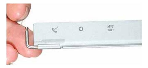
4. When installing the replacement I/O door, make sure each L-shaped pin threads through the top case, inner clutch mount, spring, and plug.
