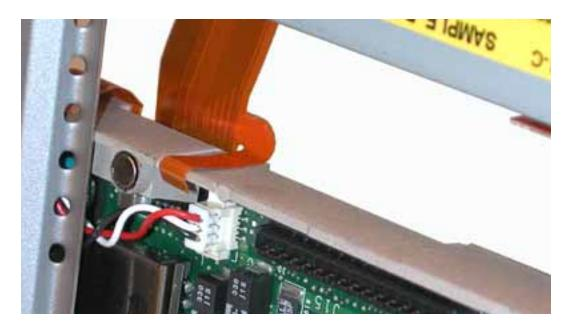
3. **Important:** With the bottom case removed, be careful when turning over the computer. Some components could become loose and fall out.
