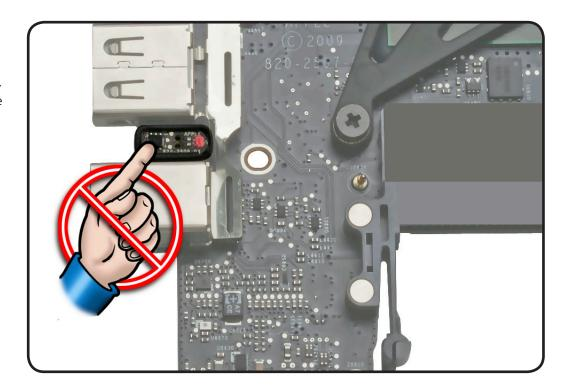
**3** Push logic board to port side first; make sure ports align; then lower board.
