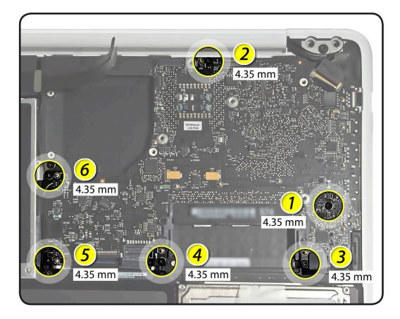
**3** Tilt up end of logic board closest to optical drive.
