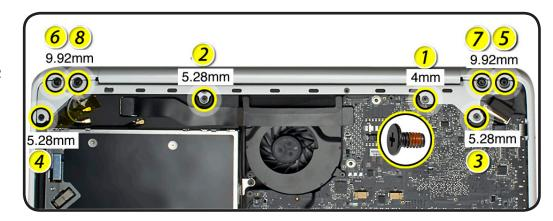
Important: Replace screws like-for-like. The screw in location 1, shown above, differs depending on the computer's manufacturing code. Replace like-for-like, as indicated in this table:
