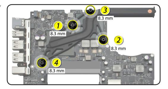
**2** Keeping heatsink parallel to logic board, gently wiggle heatsink to loosen bond to board.
