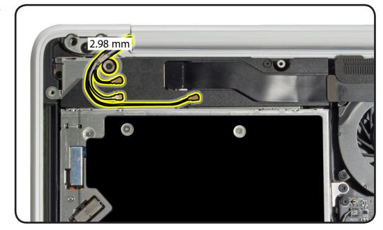
4 At LVDS cable remove gasket, peel up black tape over locking bar, and disconnect LVDS cable (image shows cable already disconnected). Pull the cable, not the locking bar.
