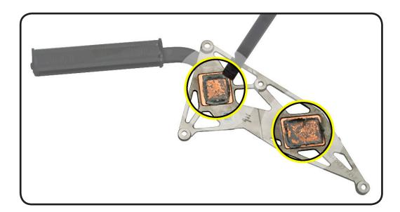
Repeat step 3 for chips on logic board.
