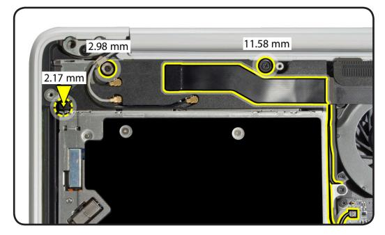
2 Without straining antenna cables, carefully flip over speaker.
