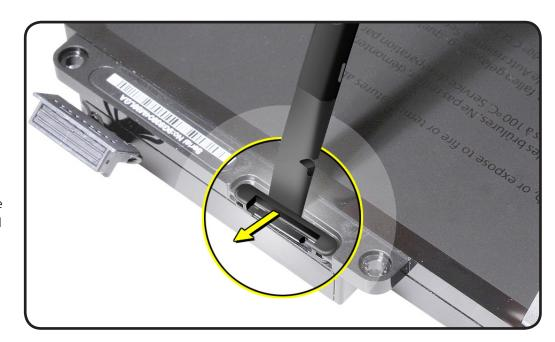
Replacement Note: All 3 snaps are identical; install flat edge into slot.
