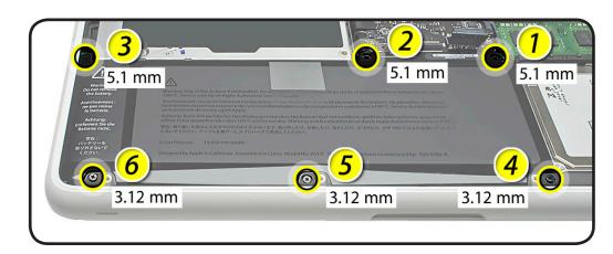
**3** If performing other repairs, be sure to leave battery cable disconnected.
