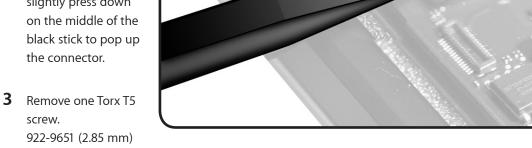
4 With your fingers, slightly lift card (< 3 degrees), and pull card to disconnect it from logic board connector.
