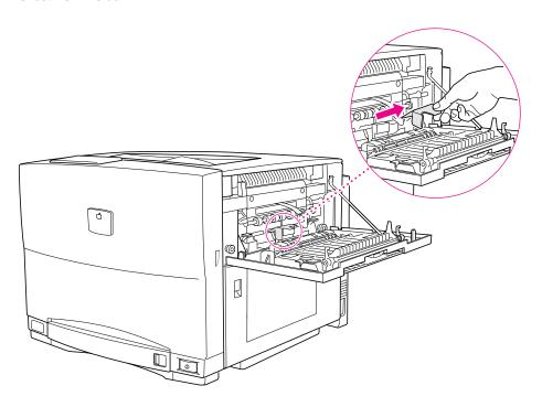
2 Open the fixing assembly and remove the oil absorption sheet from inside.
